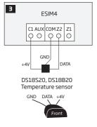
Temperature sensor wiring
